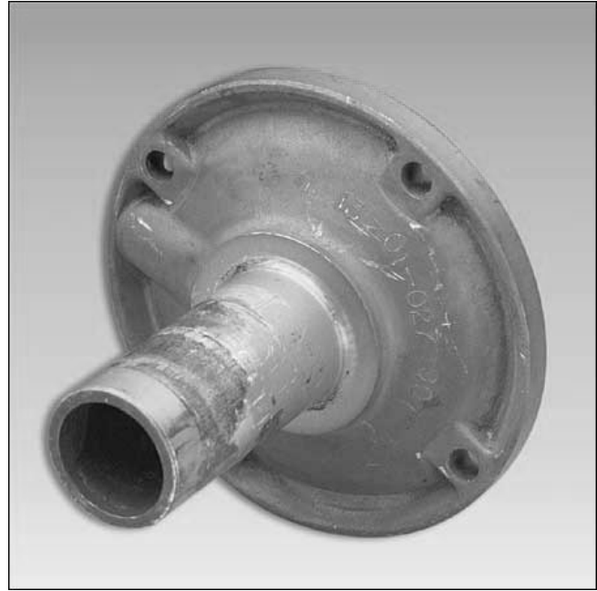
Figure 106 Worn Bearing Guide
