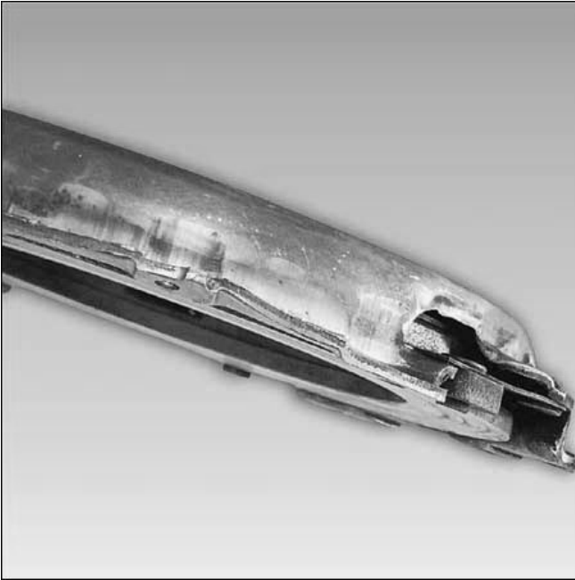
Figure 111 Bent Clutch Cover
