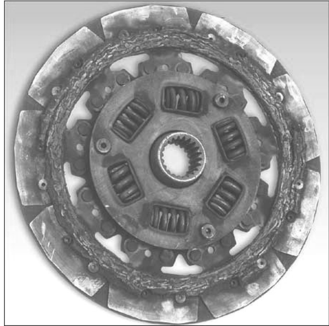
Figure 121 Burnt Friction Material
