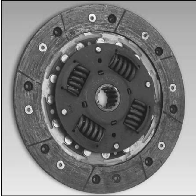
Figure 118 Worn Friction Material
