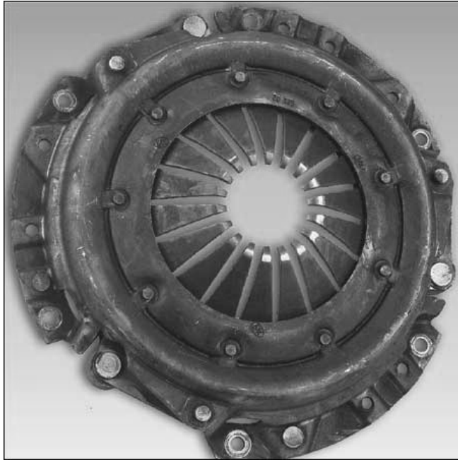
Figure 109 Contaminated Clutch Related Symptoms: Slipping. Cause: Leaking transmission or engine seal.
