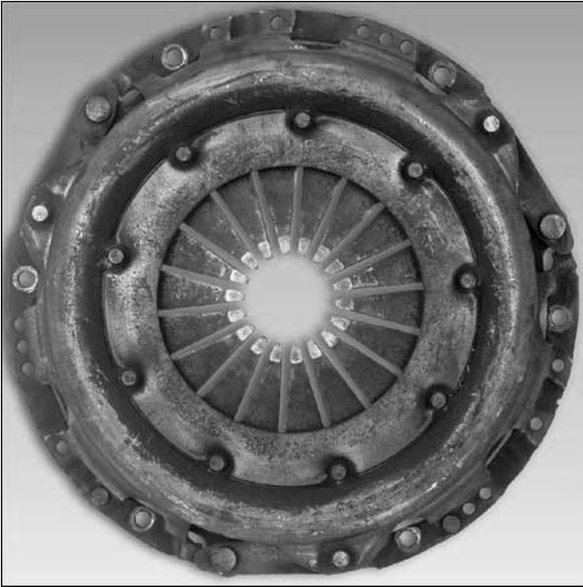
Figure 115 Excessive Finger Wear
