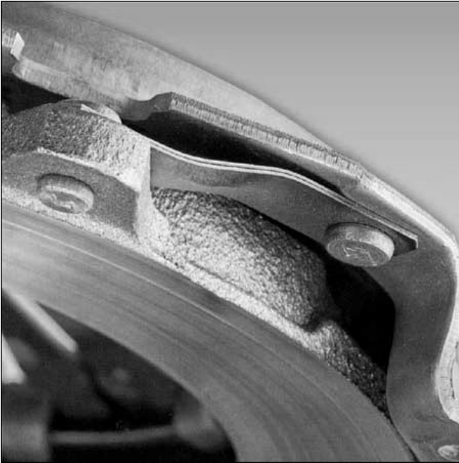
Figure 126 Bent Clutch Drive Strap Related Symptom: Chatter.
