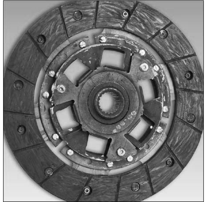
Figure 104 Broken Torsion Damper
